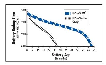
stage charging technique that increases the useful service life of UPS batteries while optimizing battery recharge time.
